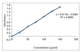
Figure 2: Calibration curve of quercetin in distilled water
