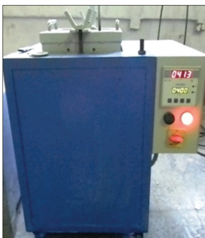
Figure 4: Kupipakwa in electric muffle furnace
