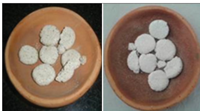
Figure 3: Pellets before and after ignition in furnace method
