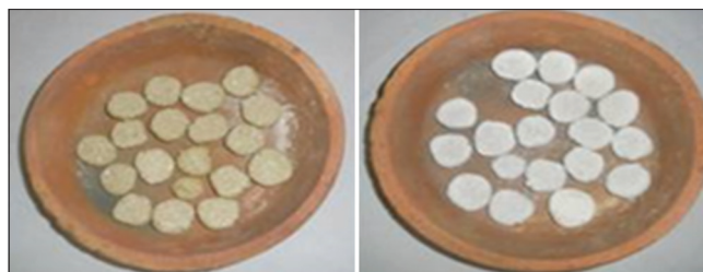
Figure 2: Pellets before and after ignition in classical method
