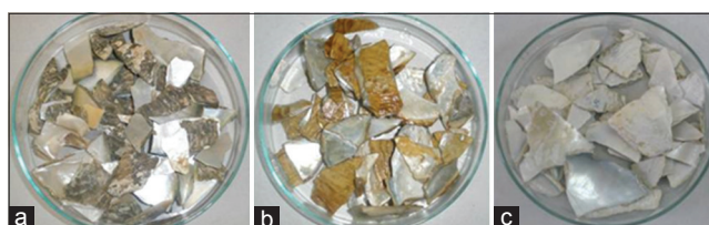
Figure 1: (a) Raw Sadaf before purification. (b) Sadaf after boiling in Sirka. (c) Sadaf after washing in hot water
